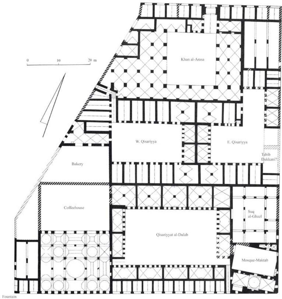
Fig. 12. Complex of İpshir Pasha. Groundplan showing structures' functions. Based on: David, Waqf d'İpshir Paşâ , Pl. 16.
